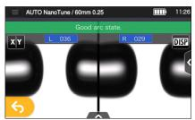
When the splicer shows "Good arc state", prepare fiber again to proceed to the splicing process. \*Fibers are not spliced in the arc test.
