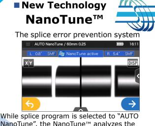
NanoTune", the NanoTune™ analyzes the cleaved fiber surface and then sets up optimal splice condition.
